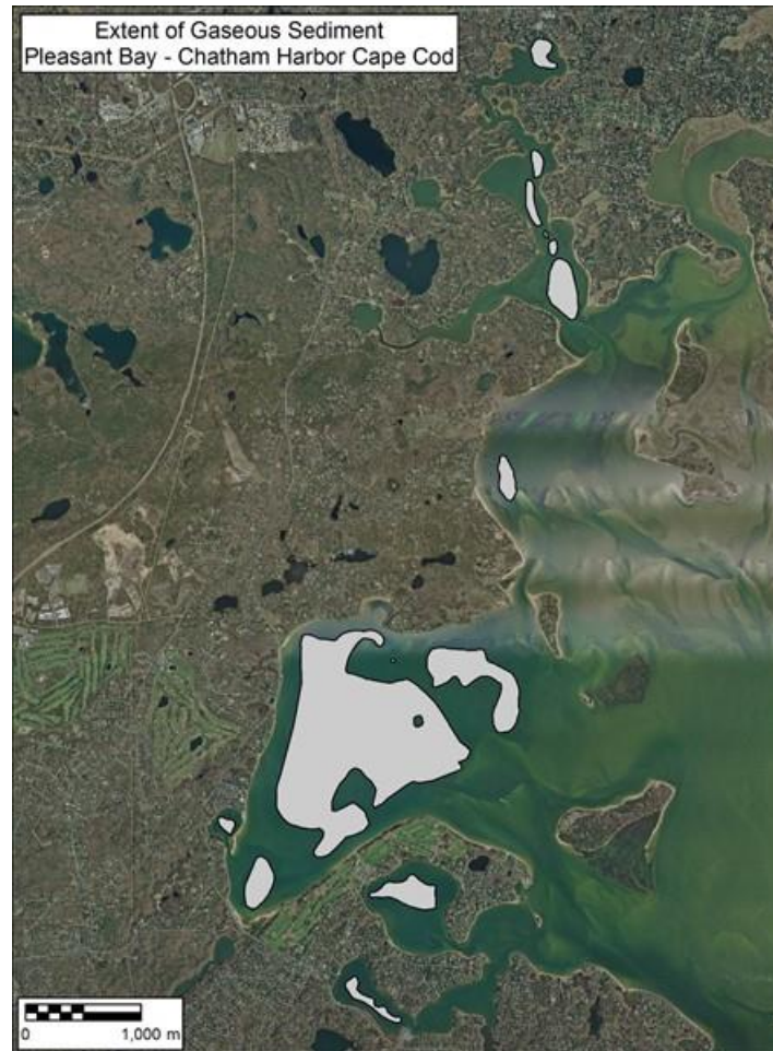
Figure 1.29. Map of Pleasant Bay showing the extent of gaseous sediment. 2014 USGS Digital Orthophotograph Basemap ( www.massgis.gov ). North is towards the top of the page.
