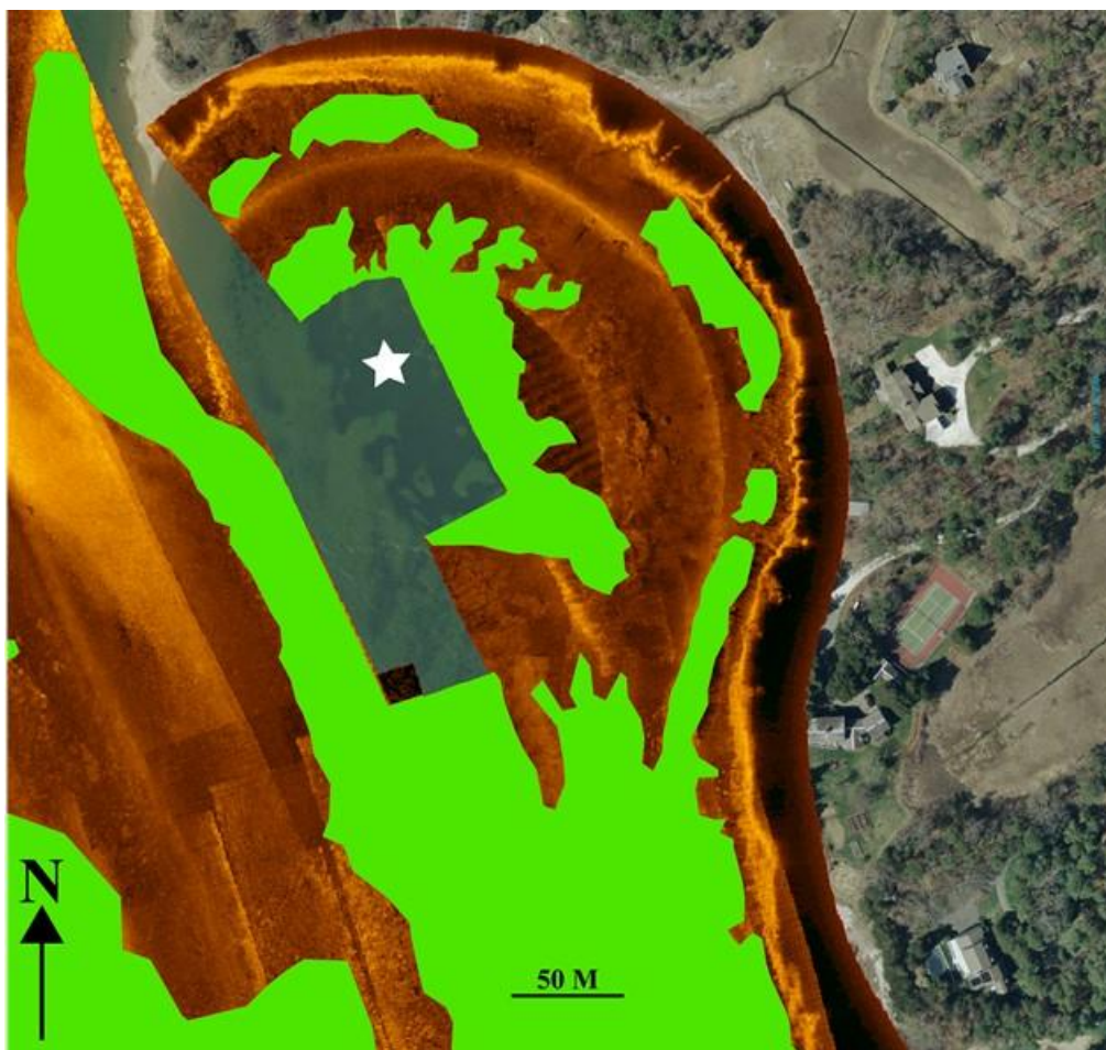
Figure 1.26. Example of eelgrass mapping near Barley Neck. Only areas with sidescan sonar coverage were included. Green polygons are areas where eelgrass is present in patches >100 m 2 . The white star is in an area of likely eelgrass beds but was not included as no sidescan imagery was collected in that location.
