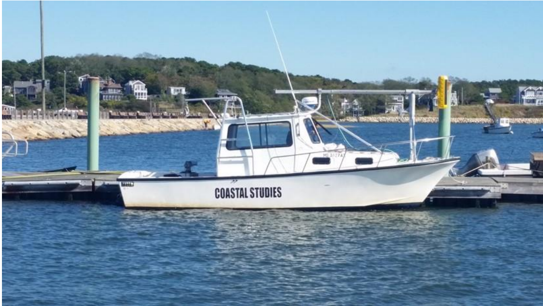
Figure 1.3. The R/V Marindin, a modified Eastern™, 8.2 m LOA, with a 2.6 m beam and a 0.61 m draft. The Edgetech 6205 is pictured on the custom-designed and built mounting gear
