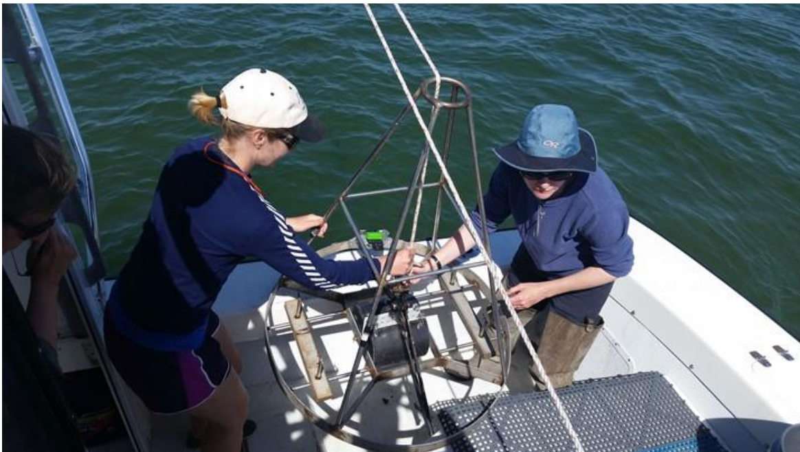
Figure 1. 4. Young-Modified Van Veen grab sampler. C.G. Kennedy and Dr. M. Tyrrell Pictured onboard the R/V Marindin
